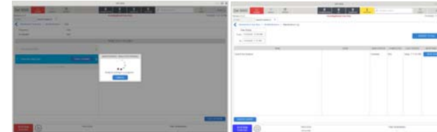
Figure 8 Examples of a wizard used for routine maintenance. Wizards can run automated diagnostic and maintenance routines, such as priming or cleaning (left). When maintenance is completed through a wizard, the task completion is automatically recorded in the maintenance log (right).
