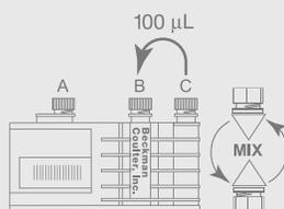
For P/N 442745 (2 x 300 tests): Quantitatively transfer 100 microliters (0.1 mL) of the contents from the smallest compartment (C) into the center compartment (B).
