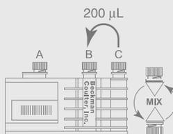
For P/N 476861 (2 x 400 tests): Quantitatively transfer 200 µL (0.2 mL) of the contents from the smallest compartment (C) into the center compartment (B).
